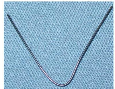
The Nickel and Titanium *atoms* in the Nitinol wire are in an ordered arrangement, or *crystal structure*. But nothing's perfect. There are mistakes in the way the atoms are arranged, and these mistakes are called *defects*. These mistakes could be missing atoms, or extra atoms that are trapped in there. When this kind of
