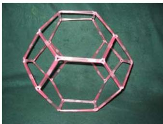
Congratulations! You have completed your zeolite model! In this model, the silicon and aluminum atoms would be where the bendy parts of the straw are. The oxygen atoms go on in the middle of the long part of the straws. If you want, you can cut out different colored circles from paper and place them where the atoms go.
